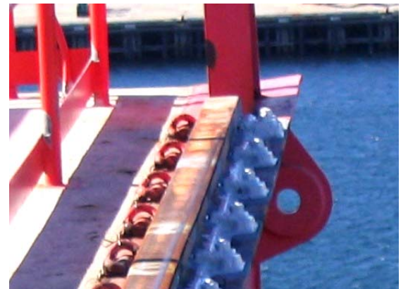
Top: A single cleat and pigtail prior to coating Above: Cleat and pigtail after being coated with Enviropeel Right: A length of track on the jib showing coated cleats linked with Enviropeel to improve security Below Right: Views of Enviropeel coated cleats
